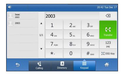
3. Press or tap the **Transfer** soft key to complete the transfer.
