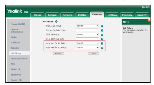
3. Select Enabled from the pull-down list of Audio Alert for BLF Pickup.
